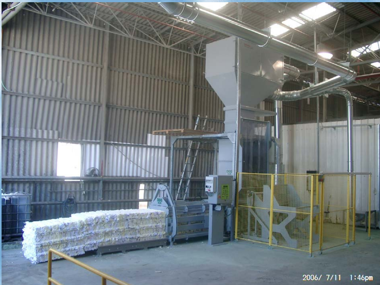
Feeding of automatic horizontal baler from air separator and from tipping device No dust outside the system. No dust handling nor dust disposal!
