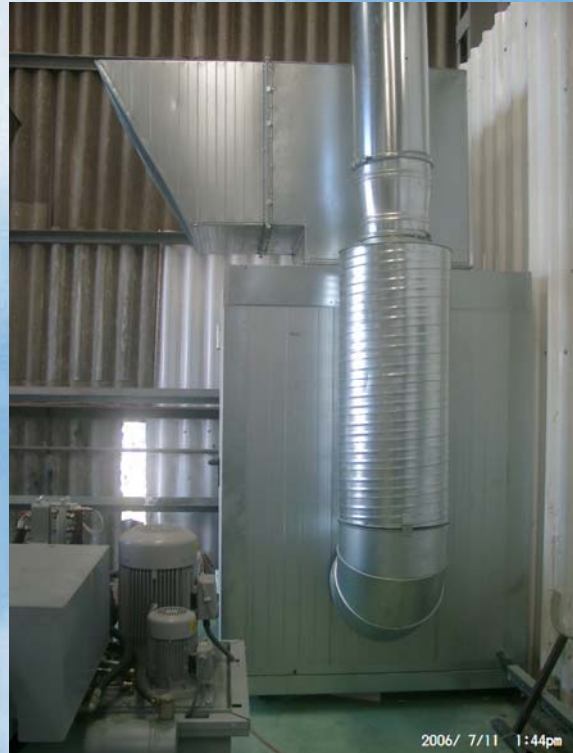
8. Acoustic cabinet for the vacuum unit. Noise level is reduced to 72 DbA
